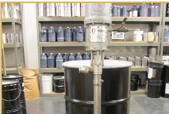
A 10:1 airless transfer pump is recommended for pumping the BGA out of drums.
