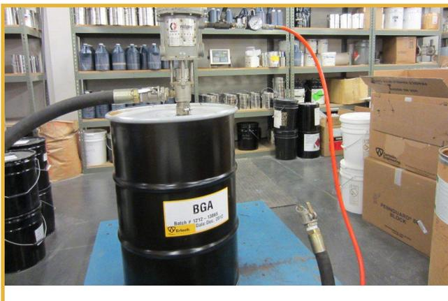
Pump mounted down on scale.
